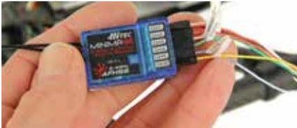
**6. Receiver Installation.** Secure your receiver to the upper frame using hook and loop tape and secure the antenna wire(s). Note that only low-profile end pin receivers are suitable for the Crossfire due to the close proximity of the fuselage shell when fitted.
