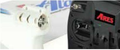
18. Remove the canopy, unplug the Li-Po battery and switch OFF the transmitter. Slide the propeller over the motor shaft, position the Allen screw directly above the flat section of the shaft and securely tighten it.
