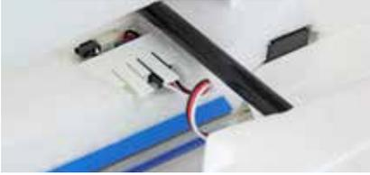
6. Slide the left-hand wing panel onto the carbon spar. Connect the servo lead as before and push the panel firmly home.
