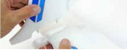
2. Position the fin and stabilizer assembly in its molded recess at the tail end of the fuselage.
