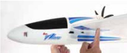
20. With the throttle stick in the low position, switch ON the transmitter once more and connect the battery to the ESC whilst keep well clear of the live propeller. Refit the canopy and check once more that the control surfaces move in the correct manner. Your Alara is now ready to fly.
