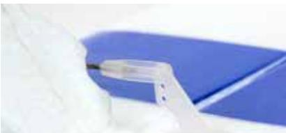
13. Now connect the aileron clevises to the outer hole of each control horn and note, again, that you may have to screw the clevis in or out to ensure that the control surface remains in the neutral position.
