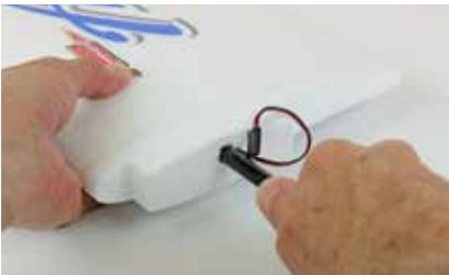
5. Offer the right-hand wing panel to the fuselage, plug the aileron servo lead into its female fuselage socket and ensure the lead-lock catch is engaged. Push the wing panel home.
