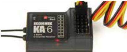
3. Pairing will be complete when the receiver's fast-flashing red LED turns solid red. You should now have full control of your Alara. Reboot the system by switching the receiver OFF then the transmitter, and switching back on again, transmitter first.
