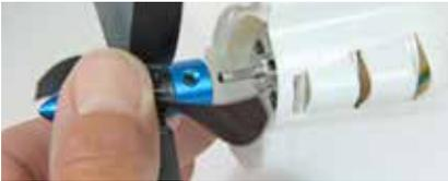
19. Check that your Alara sits level when balanced on either side of the fuselage at a point 65 – 70mm back from the leading edge. Adjust the position of the battery to ensure that the balance point is achieved.
