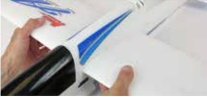
7. Insert one M3 x 10mm machine screw in the underside of each wing panel and tighten to securely clamp the spar. Take care not to over-tighten the screws.
