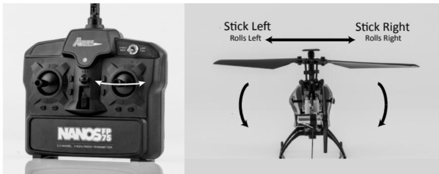
Moving the right-hand stick to the left will roll the helicopter to the left, allowing it to be flown to the left. Moving the right-hand stick to the right will roll the helicopter to the right, allowing it to be flown to the right.
