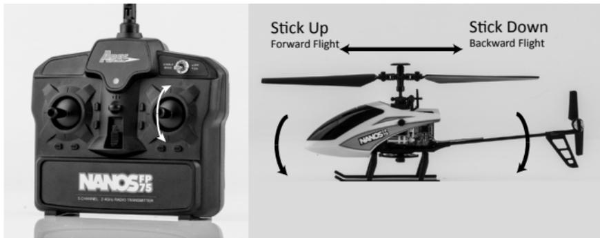
The right-hand stick controls both the elevator (pitch fore/aft) and aileron (roll) channels. Pushing the stick forward will pitch the nose of the helicopter downward, allowing it to be flown forward. Pulling the stick down pitches the nose of the helicopter upward, allowing it to be flown backwards.
